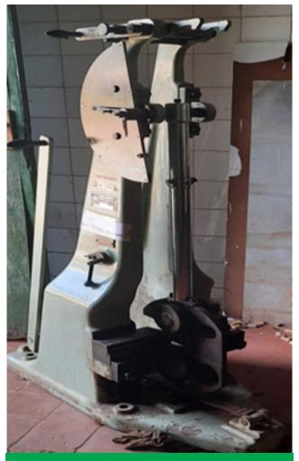
Impact testing machine (Materials Science Lab)
