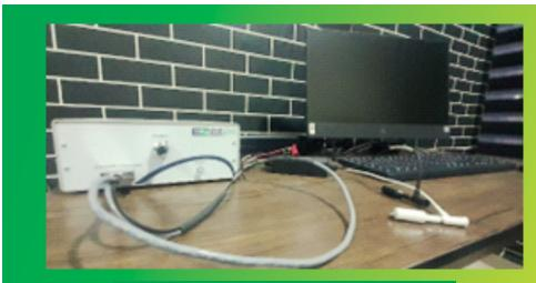
8 EZStat Pro Potentiostat /Galvanostat by Nuvant
