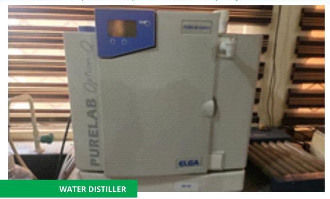
A water distiller is a critical piece of equipment in a biochemical laboratory, used to produce high-purity distilled water by removing dissolved salts, organic matter, and other impurities through the process of distillation.
