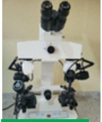
Forensic Lab, ACENTDFB, ABU Zaria Ballistic comparison microscope BestScope Analysis of Ballistic Evidence
