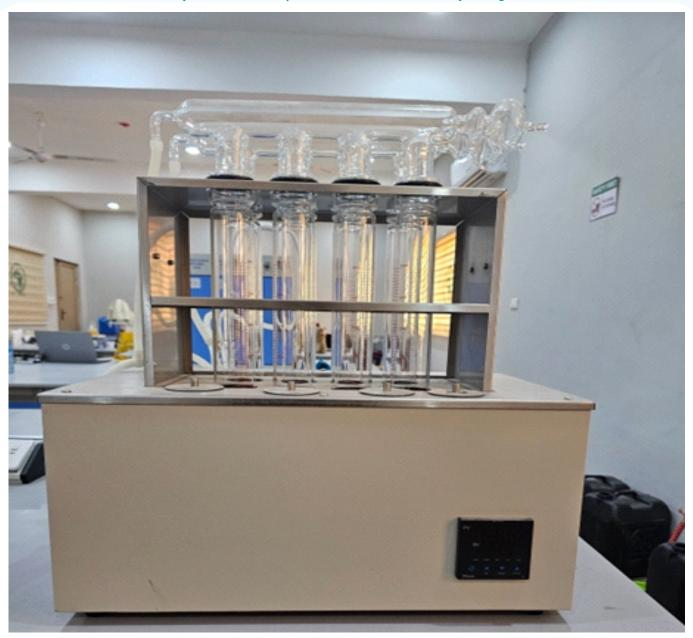
Name: Kjeldahl Digestion Furnace
