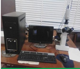
Inverted Metallurgical Microscope (NLNG Lab)
