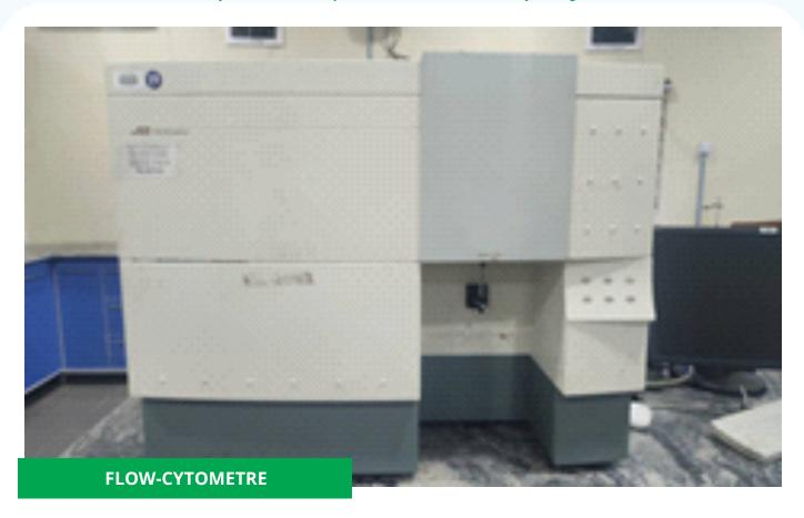
A flow cytometer is an advanced analytical instrument used in biochemical laboratories for cell counting, cell sorting, biomarker detection, and protein engineering, by suspending cells in a stream of fluid and passing them by an electronic detection system. Below is a detailed description of a typical flow cytometer, including its components, working principles, applications, and specifications.
