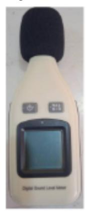
This is a digital sound level meter, also known as a decibel meter. It's a device used to measure the intensity of sound in decibels (dB).
