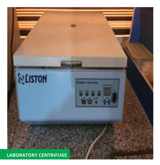
A laboratory centrifuge is a fundamental device in biochemical, clinical, and research laboratories used to separate components of a mixture based on density by spinning samples at high speeds. Here is a comprehensive and detailed description of a laboratory centrifuge used in a biochemical laboratory.
