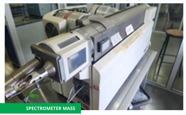
A mass spectrometer used in a biochemical laboratory is a highly sensitive analytical instrument designed to identify and quantify molecules based on their mass-to-charge ratio (m/z). It plays a crucial role in proteomics, metabolomics, drug development, and various biochemical analyses.
