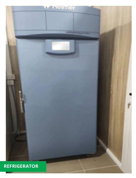
In a biochemical laboratory, a **refrigerator** plays a critical role in maintaining the integrity, stability, and viability of various biological samples and reagents. Unlike domestic refrigerators, laboratory refrigerators are specially designed for scientific use, offering precise temperature control, enhanced safety features, and proper storage conditions for sensitive materials.
