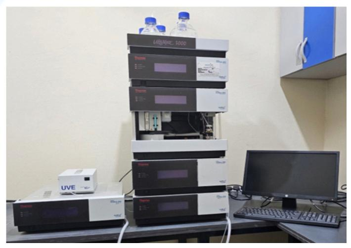
Name: Thermo Scientific Dionex UltiMate 3000 HPLC System with DAD-30000RS Diode
