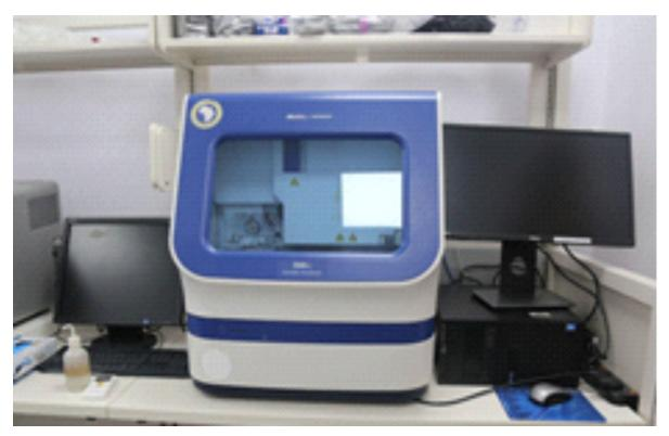
Applied Biosystems Genetic Analyser For DNA amplicon sequencing
