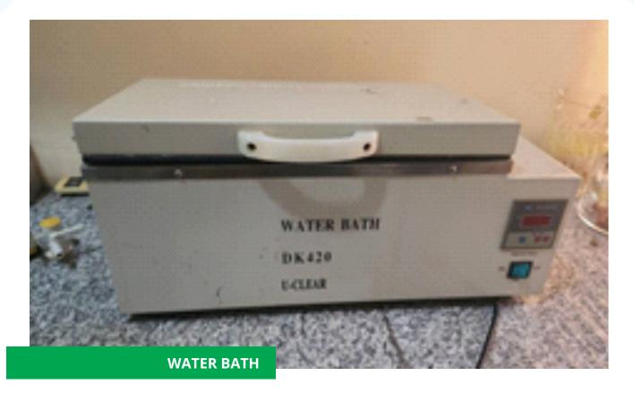
A water bath is a fundamental piece of equipment in a biochemical laboratory, widely used for incubating samples at a constant temperature over time. It provides a controlled environment ideal for many biochemical reactions and processes.
