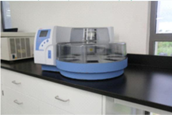
King Fisher automation system Robot for liquid handling for high throughput processes
