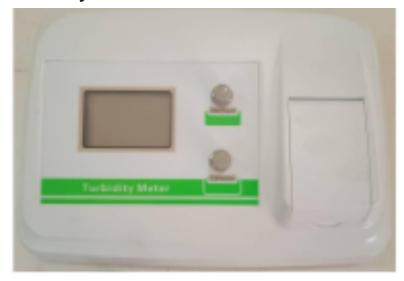
The device in the image is a turbidity meter. It is used to measure the cloudiness or haziness of a liquid, caused by suspended particles.
