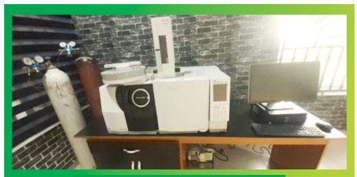
1. Shimadzu gas chromatograph with mass spec GC-MS-TQ8040
