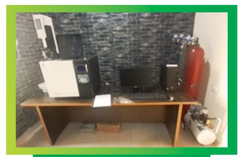
2. Angstrom gas chromatograph with flame ionization detector 8000 GC (FID)
