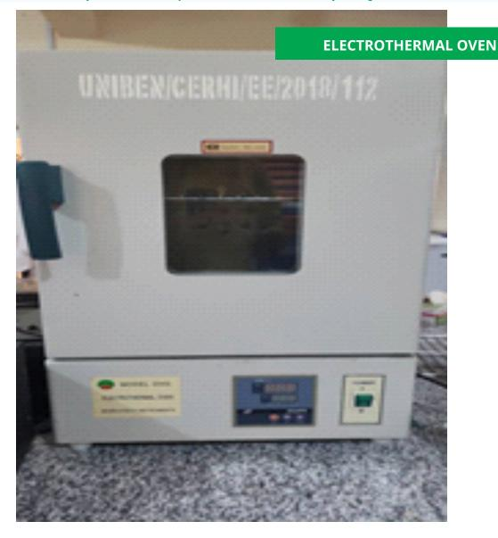
An Electrothermal Oven is a laboratory heating device that uses electric resistance heating elements to produce and maintain elevated temperatures for various drying, sterilizing, or thermal processing tasks. It is an essential piece of equipment in biochemical, microbiological, pharmaceutical, and research laboratories.
