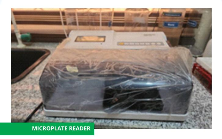
A microplate reader (also called a plate reader or ELISA reader) is an essential analytical instrument in biochemical laboratories used for quantitative detection of biological, chemical, or physical events in microplate format (96-well, 384-well, etc.). It automates and streamlines assays such as ELISA, protein quantification, enzyme kinetics, nucleic acid quantification, and cell viability.
