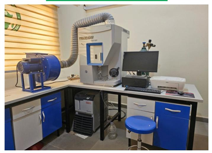
**Name:** Thermo Scientific iCAP PRO Series Inductively Coupled Plasma-Optical Emission Spectrometry (ICP OES) Systems (Thermo Fisher Scientific)
