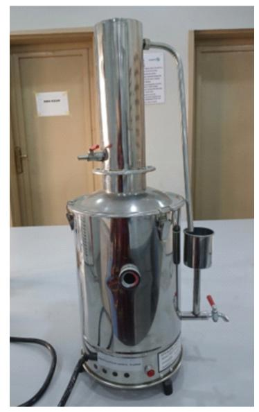
**Name:** Stainless steel distillation apparatus used for producing distilled water or other liquids
