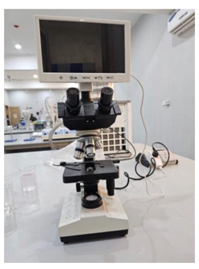
**Name:** Digital Trinocular Microscope with built-in-LCD Screen AmScope brand (XSZ-107BN model)
