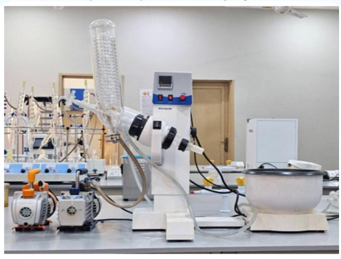
Name: Rotary evaporator (Bioevopeak)
