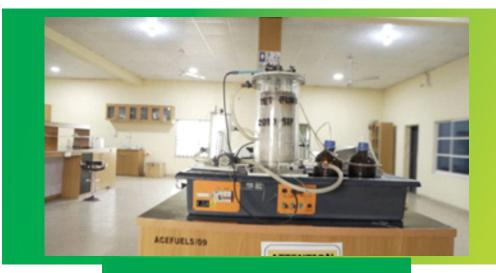
20 Tubular Stirred tank reactor
